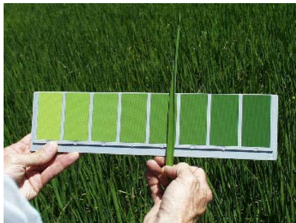
Figure 1. A rice leaf is compared to the UC leaf color chart to estimate N content.
